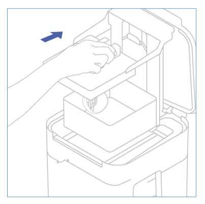
**ALTERNATIVE WASH METHOD** Parts can also be washed in the basket, either as an alternative or in addition to the platform mount. Place parts directly in the basket after removing them from the build platform using the removal tool, scraper, or flush cutters. The basket comes installed in Form Wash. Without a build platform installed, the basket can be removed by lifting vertically from the basket mount.
