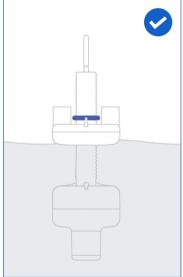
TIP The hydrometer is designed to work with 90% IPA or higher and will not work with IPA less than 90% nor any alternative solvent. After calibrating in fresh IPA, the hydrometer will only be effective for measuring IPA of the same concentration. The hydrometer can also be calibrated in a smaller container of fresh IPA.
