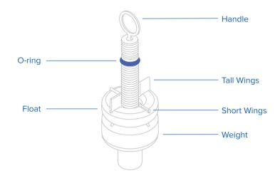
To calibrate the hydrometer, hold the handle and release the tool in the wash bucket's fresh IPA. Slide the O-ring along the ribbed stem until the O-ring aligns with the short wings at the top of the float. Leave the O-ring in this position. The alignment of the wings and O-ring will be used to check the resin concentration of IPA between washes. Store the hydrometer in the tool storage.
