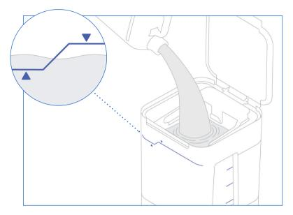
Isopropyl alcohol (IPA) is a solvent used to remove uncured resin from SLA 3D prints. Open the outer lid. Pour or siphon to fill the wash bucket with IPA to reach a level between the minimum (7.8 L) and maximum (8.6 L) fill lines. For more information about using a siphon, see *Changing the IPA* on page 9.
