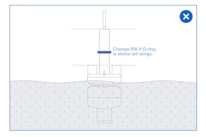
As the IPA resin concentration increases, the weight will float higher, and the stem and O-ring will rise. For a smooth, dry surface finish, replace IPA when the O-ring rises above the float's tall wings.
